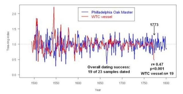
**Figure 4**. Comparison of the ring-width index of the World Trade Center vessel oak chronology (19 samples cross-dated) against the Philadelphia area oak master chronology based on living trees and independent archaeological samples. The Spearman rank correlation between the series (r=0.47) is highly significant (p<0.001) with an overlap of 280 years. This strong match suggests that the origin of the oak logs used in the World Trade Center vessel was from the Philadelphia area.
