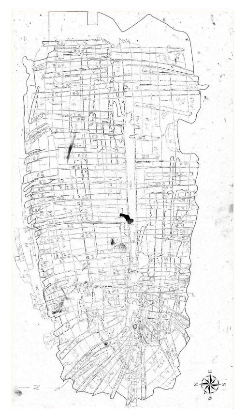
Figure 2 - World Trade Center Ship: Frame and Planking Composite of Field Sketches
