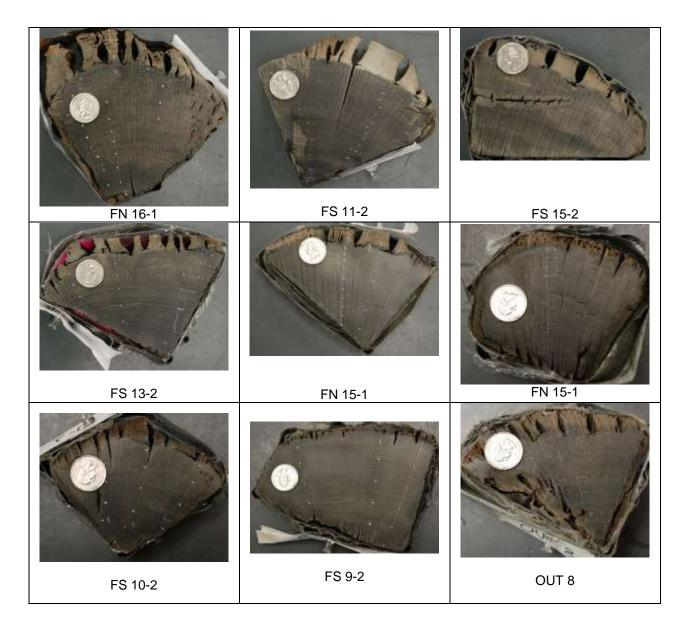
**Figure 1**. Photographs of the 23 WTC vessel timber samples analyzed by tree-ring analysis. Refer to **Table 1** for the wood species and dates of the samples.
