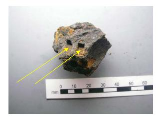
*Figure 8 - WF10S-017: Concretion with 2 square nail holes*
