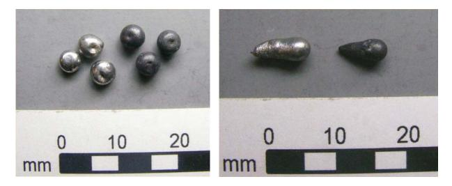
*Figure 4 - Experimental shot to the left and WTC shot to the right*
