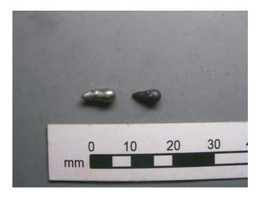
Figure 7 - Experimental shot on left and actual shot on right
