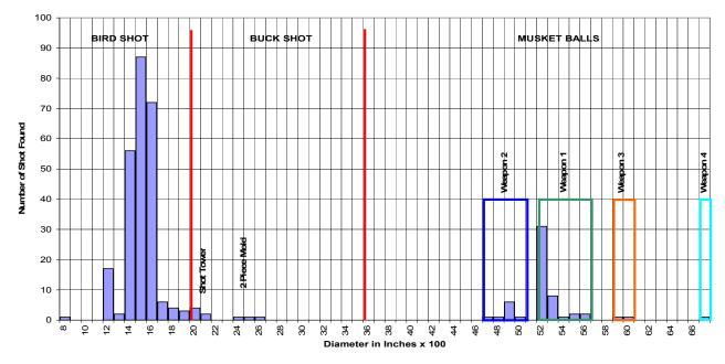
Figure 3 - Lead Shot Sizes Found on the Ship Excavated at the World Trade Center Site
