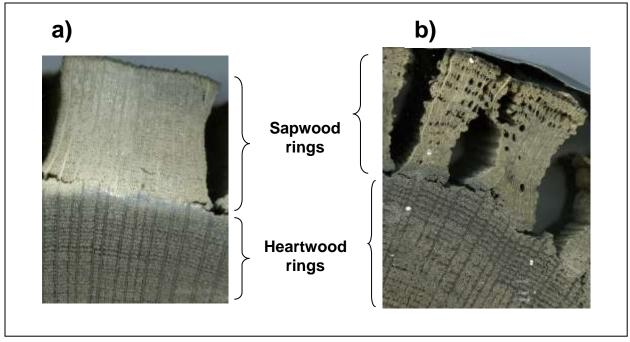
**Figure 2**. Detail of collapsed (a) and expanded (b) sapwood rings which hindered the exact dating of the last available tree rings. The outer rings of FN 16-1 are shown in (b).
