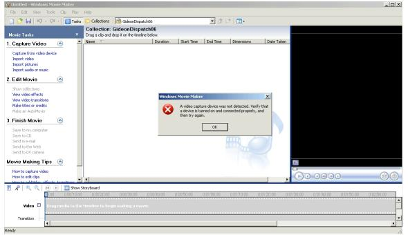
If this error occurs, check the USB connection and check to see that the Logitech Drivers have been installed. Also, if a system restart has not been completed since driver installation, this would be a good time to restart the computer.
