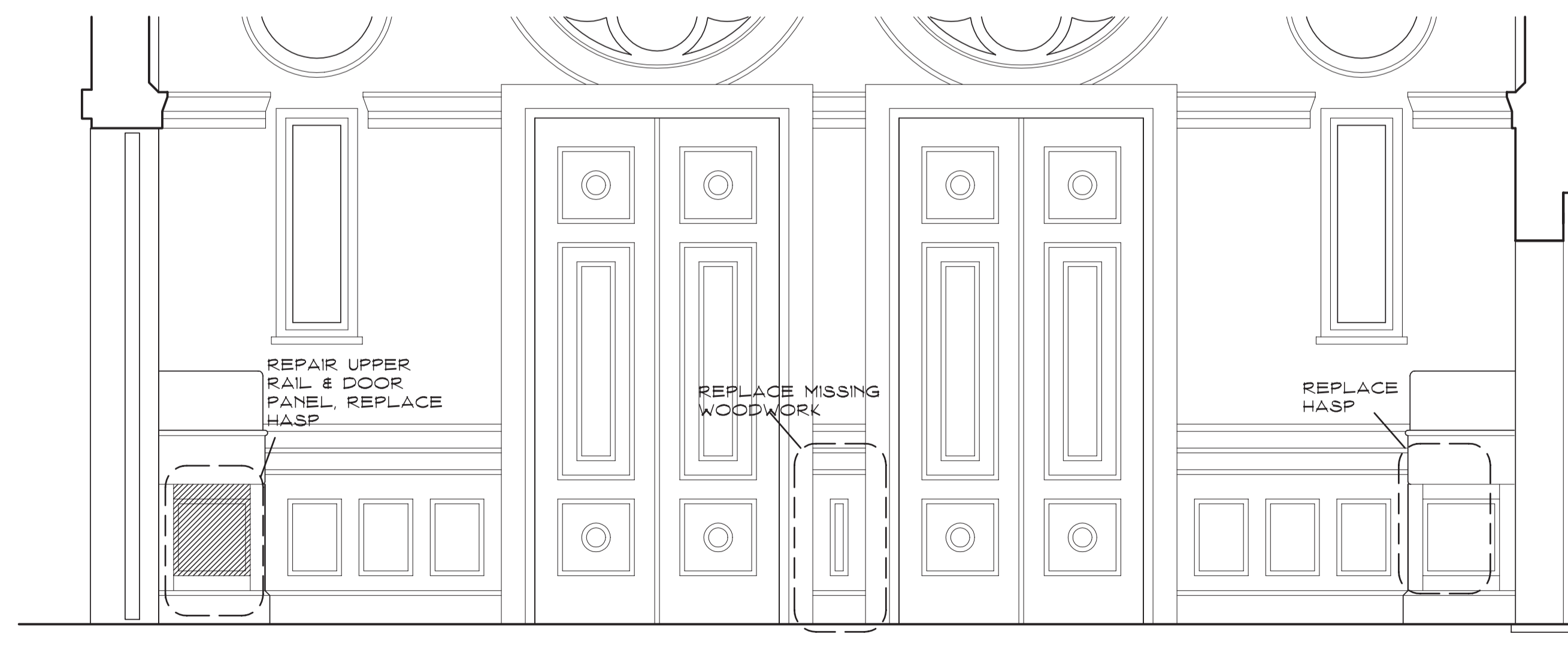
2A MAIN LOBBY, INTERIOR ELEVATION, WEST SCALE : 1/4" = 1'-0"
