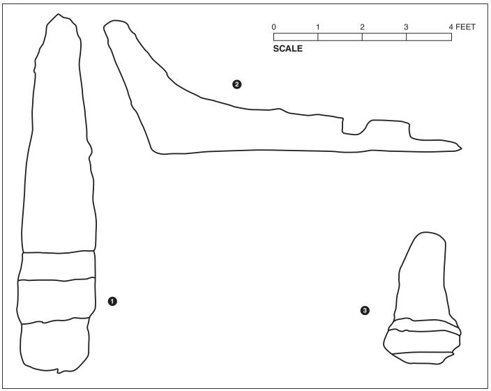
Top (1), starboard side (2), and forward side (3) views of stern knee. Images created using *Photo Modeler Scanner* and *Rhinorceros*
