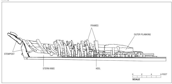
Profile view of starboard side of stern at the keel
