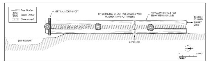
Profile drawing of east face of landfill retaining structure north of ship remnant
