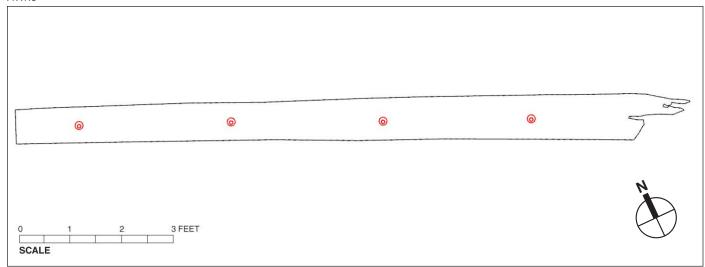
Schematic of top of keelson with nails marked in red. Image created using Photo Modler Scanner and Rhinoceros
