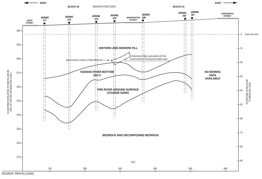
NOTES: This profile was generated using selected soil boring logs. In some cases, soil levels observed in the borings have been combined. This profile therefore represents an estimate of what the general profile of the site may have looked like and has been simplified for the purposes of this analysis. Vertical and horizontal scale are different.
