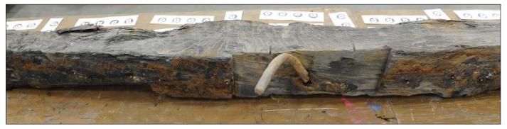
Frame FNFS 23-0 showing a mis-hit iron pin in center. Two marks on aft face of frame correspond to location of keel. Photograph by Drew Fulton
