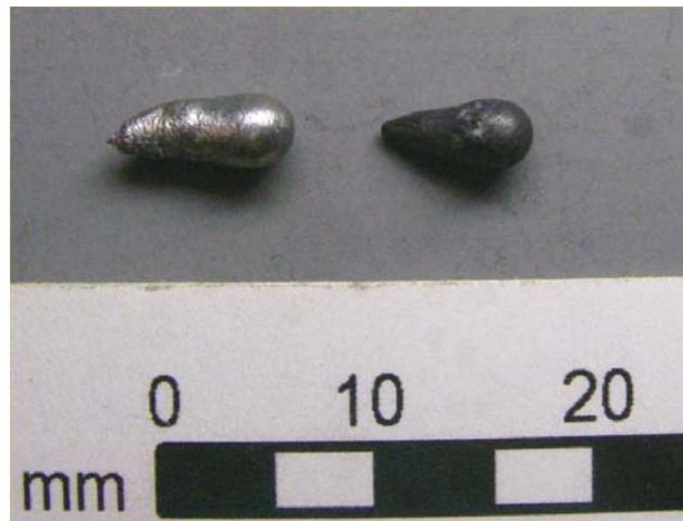
*Figure 5 - Experimental shot to the left and WTC shot to the right*
