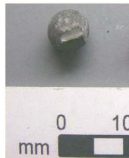
Figure - buck shot with sprue cut (WTC-USP-006-1)
