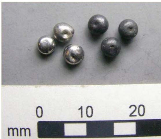
*Figure 4 - Experimental shot to the left and WTC shot to the right*
