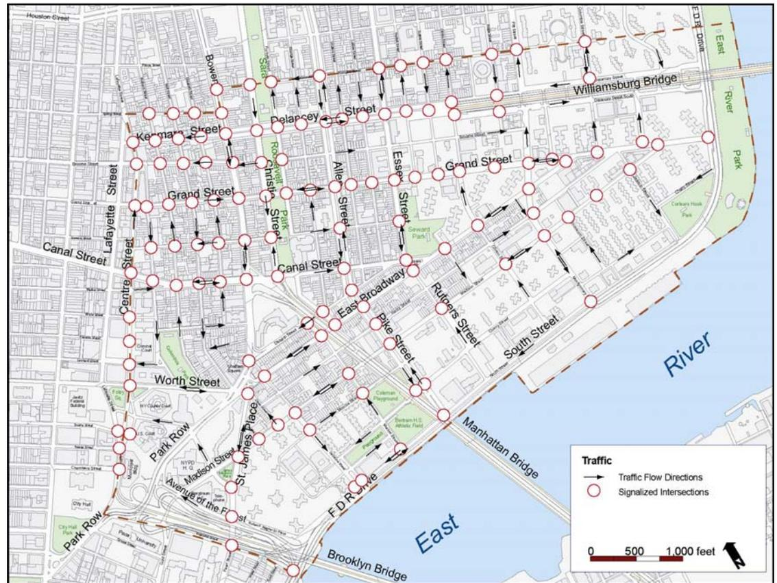
**Figure A-5: Traffic Flow Directions and Locations of Traffic Signals**
